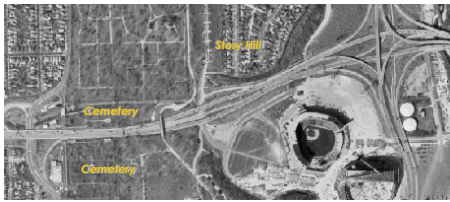
ABOVE: Photos taken in 2000 show the lack of available land from Miller Park to Howley road on which to build new freeway lanes. SEWRPC's "solution" is to double-deck the freeway in this area. The cost would be $3.4 billion and require no additional right-of-way.
