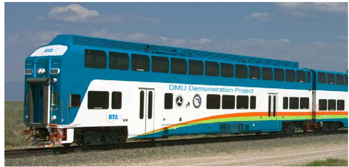
A bi-level, diesel-multiple-unit car, also known as a DMU or self-propelled coach.
